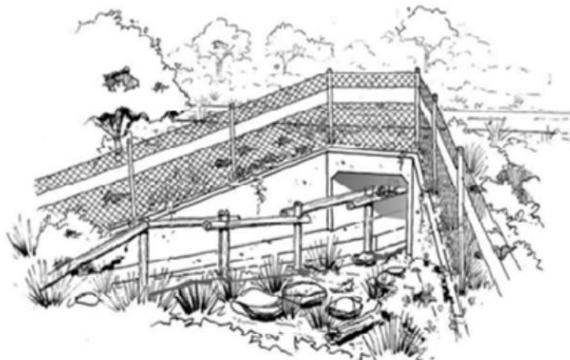
Figure 6: A simplified entrance drawing with dry passage and furniture design for koala (from TMR's Fauna Sensitive Road Design Manual, Vol 2). Note: The underpass provided along the northern access road will be larger than that shown here as it will also be designed for macropods.
